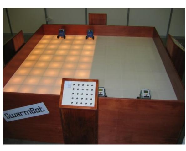
for artificial ethology. ARS is a platform of 2\*2m, divided in 10\*10 cells and surrounded by a wall 30 cm high. Every cell contains a lamp that can be turned on and off by an external console. This configuration permits to create quite easily mazes, illuminating the opportune cells, of different complexity. The visitors can interact with a team of 4 robots. These robots have 2 infrared sensors (pointed toward the floor to
