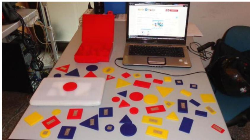
Figure 3: The Block Magic prototype that includes a tablet able to recognize each RFID tag and transmits the signal to the PC/tablet; a tablet equipped with a dedicated software and enhanced with Artificial Intelligence; 48 Logical Blocks tagged with RFID antennas
