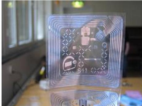
Figure 1: A typical RFID tag. The dimension of the square is in the centimeters order, with a minimum thickness
