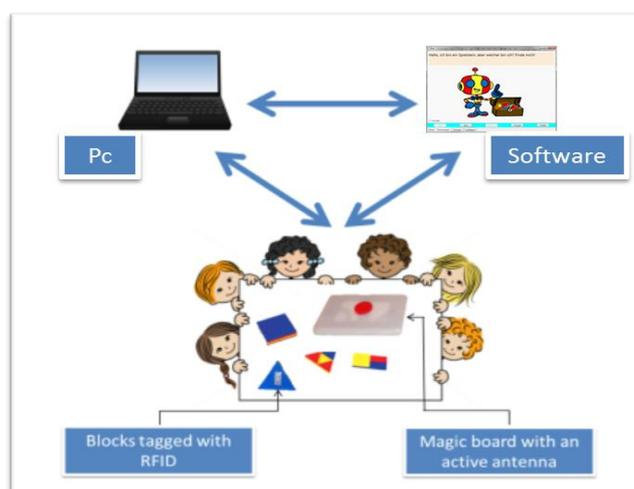
Figure 4: simplified schema of Block Magic. The children interact and use the Logical block tagged with RFID technologies and place it on a "Magic Board", an active antenna; the signal is transmitted to the PC/Tablet and the software engine proposes the appropriate exercises to the children based on the results previously collected in the session.
